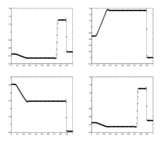
Fig. 4. Lax's problem,  $\Delta x = 1/200$ . From left to right, top to bottom, (1) density (CO-DG-hr1e-3); (2) velocity (CO-DG-hr1e-3); (3) pressure (CO-DG-hr1e-3); (4) density (CO-DG-hr1m-3).
